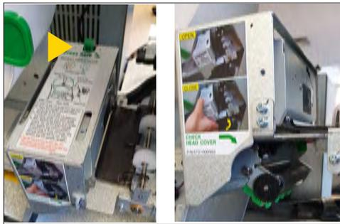
The black plastic section of the printer will now hinge backwards, remove any paper debris
